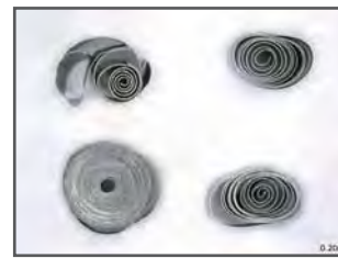
Evacuation from grooves is poor, inviting sudden breakage
