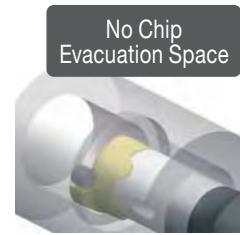
Evacuation from grooves is poor, inviting sudden breakage
