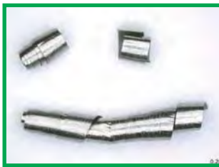
Stable and smooth evacuation of curled chips even on small bore diameters
