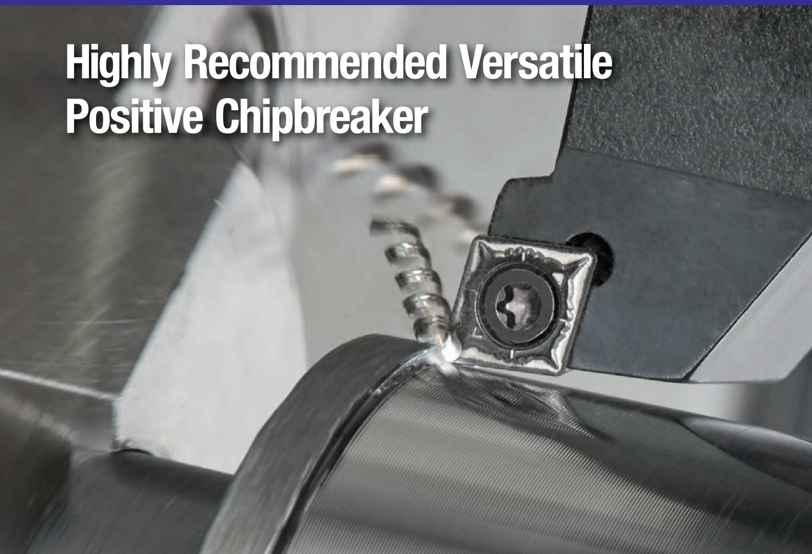
Positive GU Type Chipbreaker Application Range
