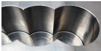
Keep the value of p_t for PDL type tools to less than 70% of the tool diameter ( \phi D_c ).
