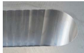
Keep the value of p_t for PCT type tools to less than 50% of the tool diameter ( \phi D_c ). For a_e , refer to the dimension under " a_e max" in the stock/ dimensions tables titled "Holders Max. Depth: 3D/5D".
