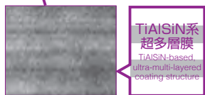
TiAlSiN系超多層膜 TiAlSiN-based ultra-multi-layered coating structure 10nm 刃先被膜断面TEM像 Cross Section of Edge Coating: TEM Image
